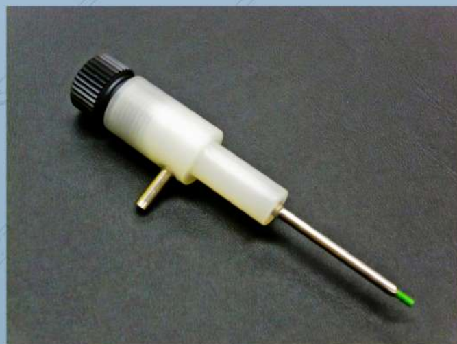
Overlook OneShot™ co-ax filler needle w/ Upchurch connector and Teflon coating
